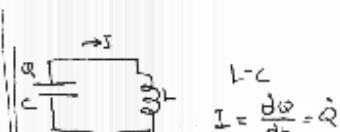
$$E = E_L + E_C = \frac{1}{2} L I^2 + \frac{1}{2} \frac{Q^2}{C} = \frac{1}{2} L \dot{Q}^2 + \frac{1}{2} \frac{Q^2}{C} \quad (1')$$
